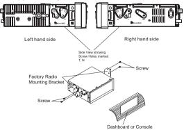
Fasten the unit to the factory radio mounting brackets. Align the screw holes on the bracket with the screw holes on the unit, and then tighten the screws (5x5mm) on each side.
